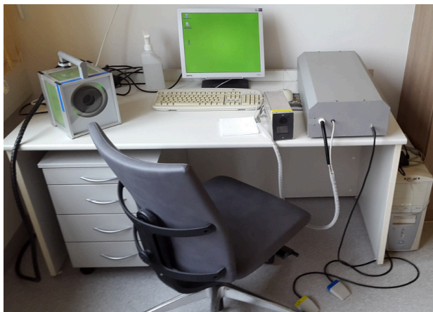
Fig. 1. Measuring station with multi-spectral camera (left) and hyperspectral probe HySkinII (right)
