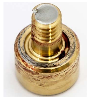
Figure 3. Torsion fracture of screw M6.
