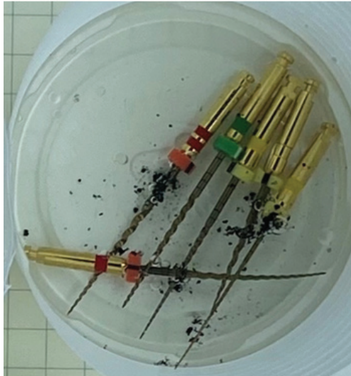
Fig. 3. Chemical load test of nickel-titanium tools COXO SC PRO
