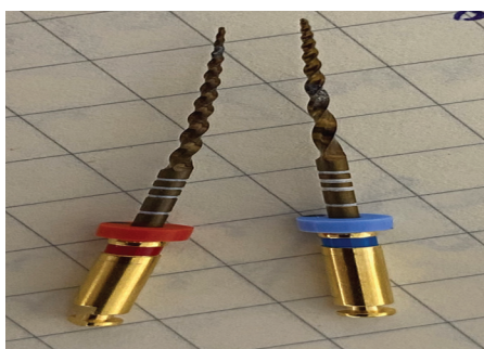
Fig. 4. Nickel-titanium tool COXO SC PRO 06/25 with no deposition in the area of the alleged breakage
