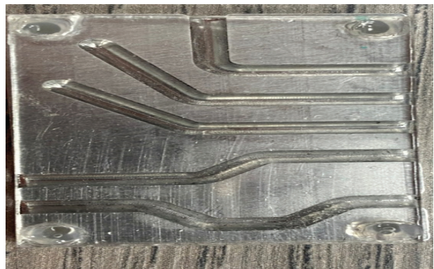
Fig. 1. Simulation endodontic unit. Dimensions 40.0 x 25.0 x 6.0mm, canal depth 2.2 mm
